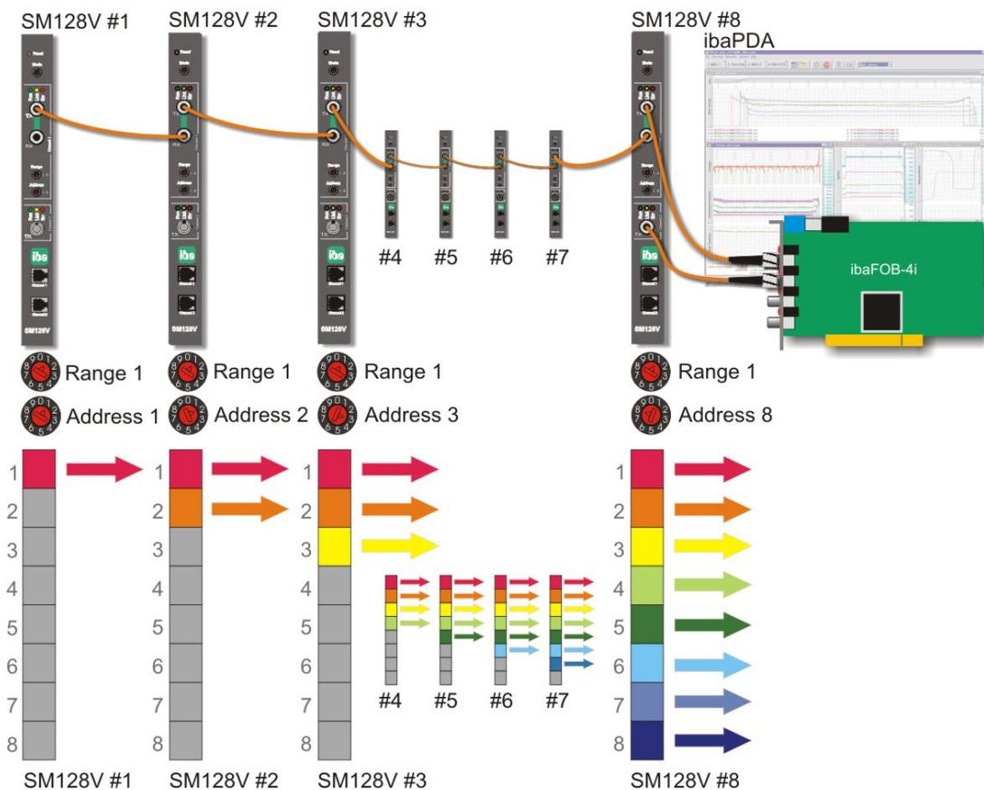
Figure 13 Cascade mode with 8 x SM128V
