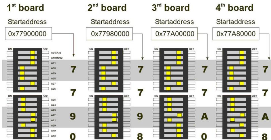
Figure 8 DIP-switch, settings for up to four SM128V cards in ALSPA C80 HPCi
