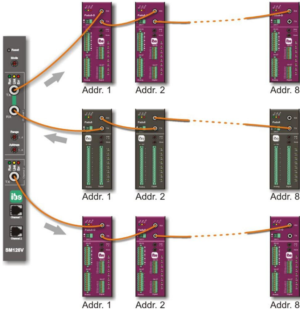
Figure 15 System topology for process i/o application with ibaPADU-8 and ibaPADU-8-O
