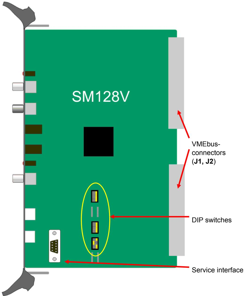
Figure 2 View on assembly side
