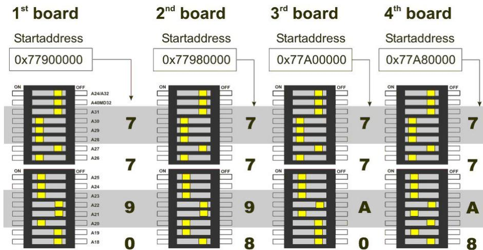
Figure 6 DIP switch, settings for up to four SM128V cards in ALSPA C80 HPC
