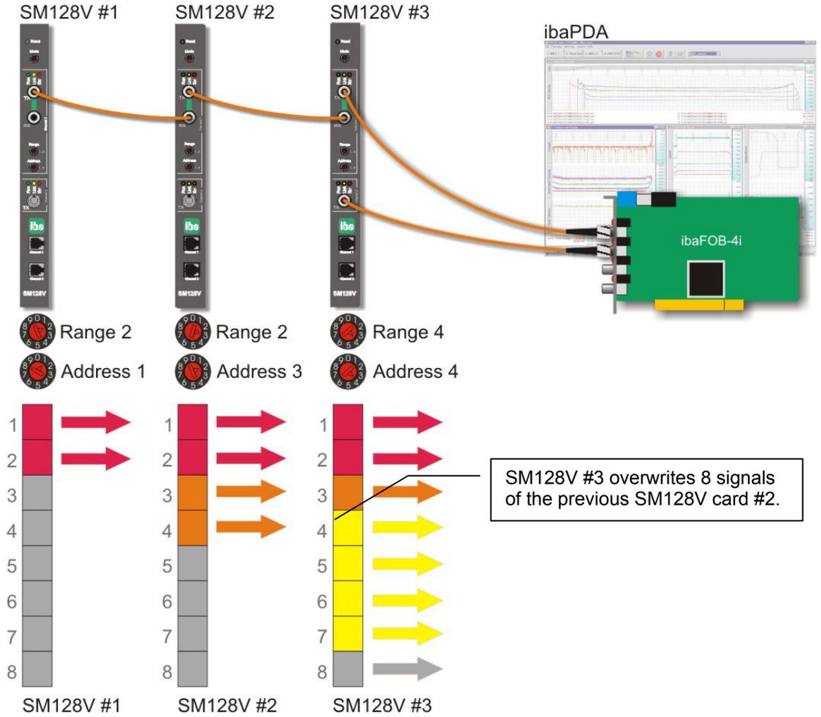
Figure 14 Cascade mode with 3 x SM128V
