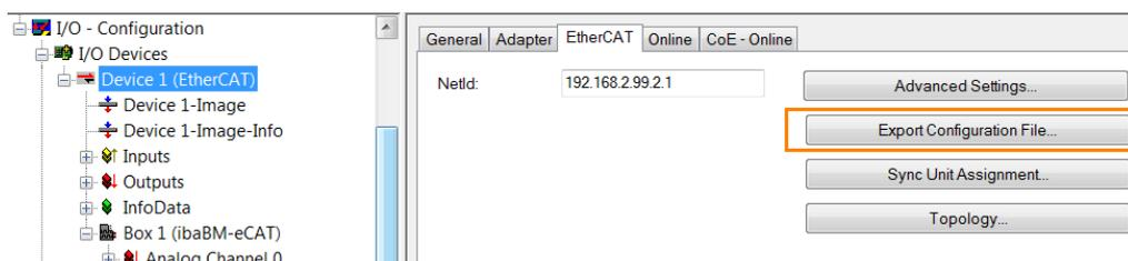
Please note, that if ibaBM-eCAT is to be used as EtherCAT SubDevice, the device must be integrated into the EtherCAT configuration before exporting (see chapter
