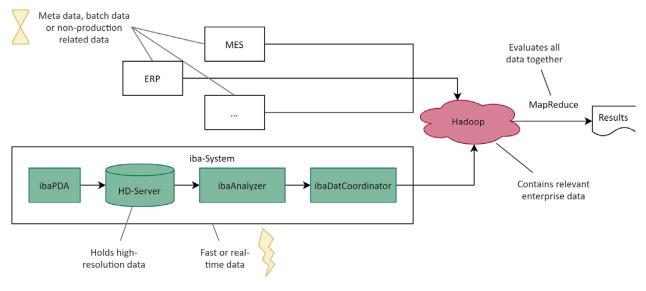
Fig. 4: Lambda architecture with the iba system as data source
