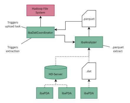
Fig. 5: Proposed solution for a connection of Hadoop to the iba system
